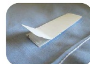
Heatsealed underneath an additional patch
